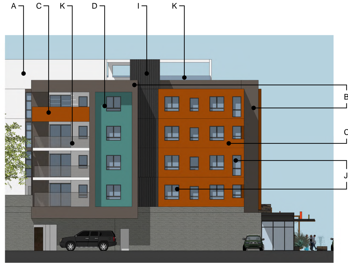
PARTIAL SOUTH ELEVATION ENLARGED WITH MATERIAL 2 1" = 10'-0"
