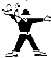
MOVE RIGHT Left arm horizontal Right arm sweeps upward to position over head
