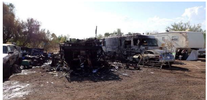
Undetermined mobile home fire with multiple potential ignition sources, to include a Dewalt lithium-ion battery fan
