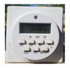
To program the timer's clock, hold down the "clock" button and adjust as needed using the "week," "hour," and "minute" buttons.
