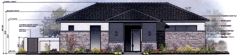
FRONT ELEVATION ELEVATION B 1/4" = 1'-0"
