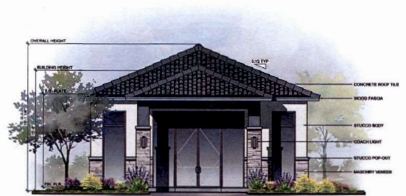
FRONT ELEVATION ELEVATION B 1/4" = 1'-0"
