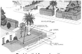
Residential fence locations (Figure 1) The fence on the street side of a corner lot adjacent to a key lot must be set back, where it adjoins the key lot, a minimum of 10 feet for a distance of 20 feet along the street (see figure 2).
