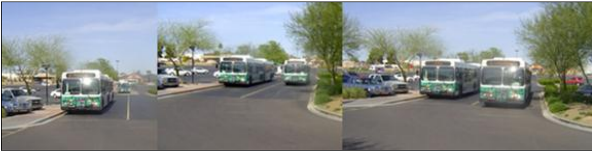
Figure 3.8 Buses that maneuver out of the pick-up/drop-off lane have no alternative available except to cross into oncoming traffic.
