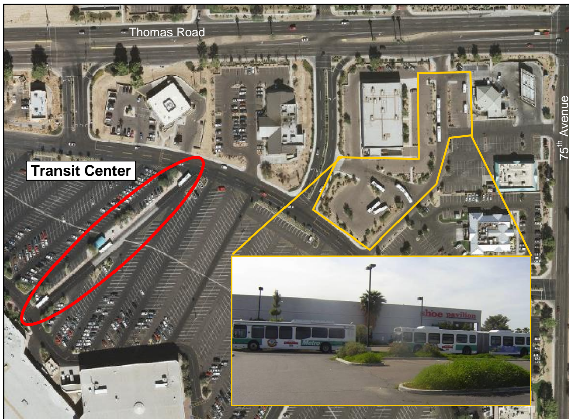
Figure 3.7 Buses serving the Desert Sky Mall Transit Center layover on private property. This aerial photo shows eight vehicles, including two articulated buses, awaiting their next routes. In the photo inset, an articulated bus and a standard 40-foot bus wait during their layover.
