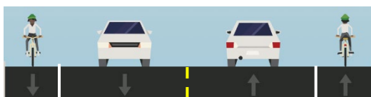
Current Travel Lanes (Parking allowed south side)
