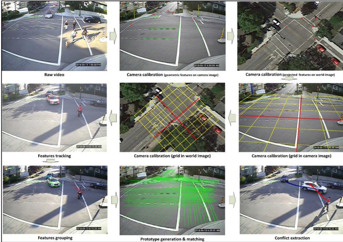
Figure 6: A Diagram of the Process of Traffic Conflict Analysis (Y. Guo et al., 2020)
