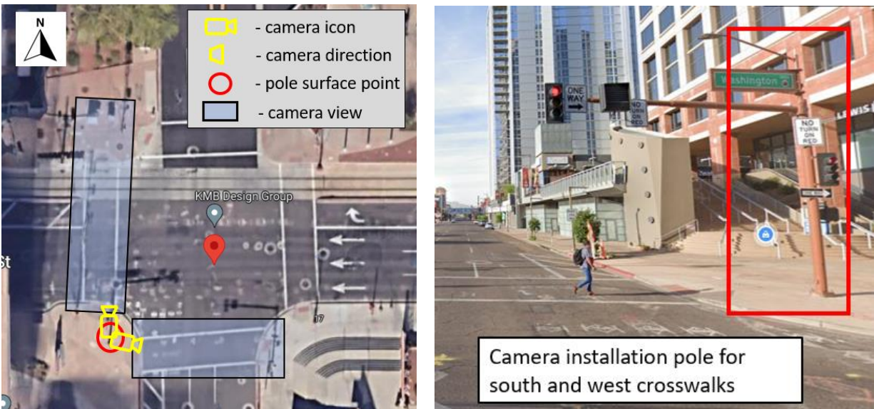
Figure 28: Example Annotated Figure of Camera Installation Positions for Washington and 3 rd Intersection.
